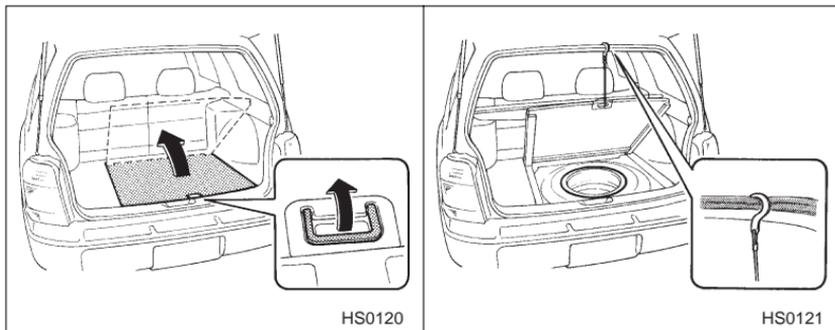
To open the lid, pull the handle up. To keep the lid open, hang the hook provided on the backside of the lid on the rear edge of the roof. The spare tire is stored under the storage tray.
