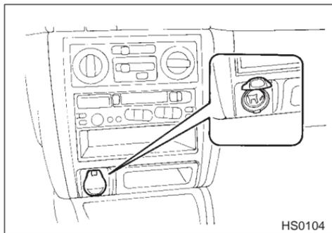
The front accessory socket is located on the lower part of the instrument panel.
