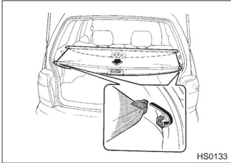
To extend the cover, pull the end of the cover out of the cover housing, then insert its hooks into the catches as shown. To rewind it, unhook it from the catches and it will rewind automatically. You should hold on to the cover and guide it back into the cover housing while it is rewinding.
