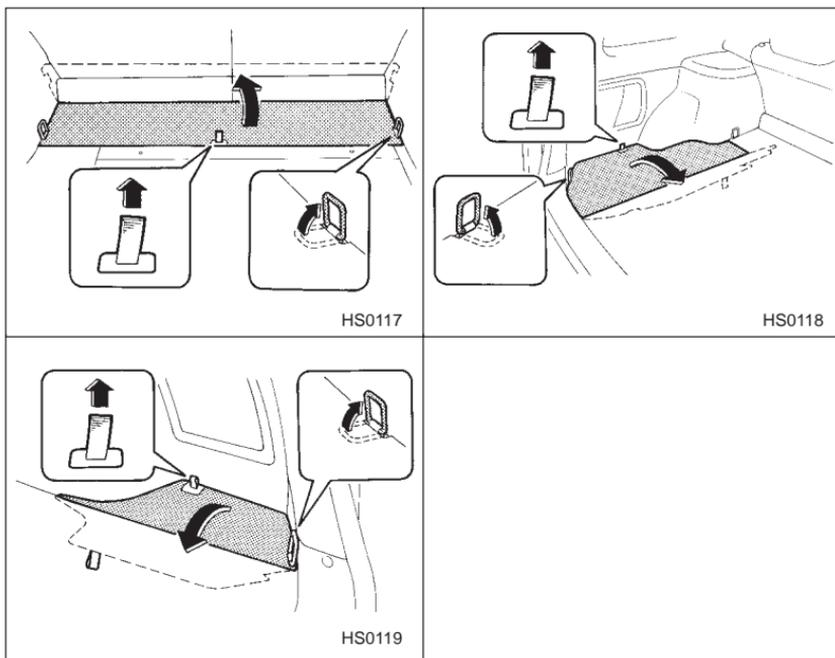
To open the lid, raise the cargo anchorage eyelets and pull the tab up. The jack and jack handle are stored in the left side storage tray.
