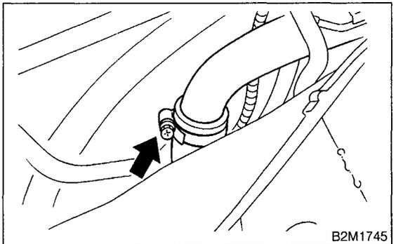
18) Remove fuel filler pipe to under side of vehicle.
