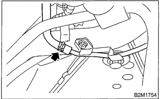
17) Loosen clamp, and disconnect fuel filler hose from fuel filler pipe.
