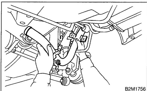
5) Connect evaporation hoses to pipes.
