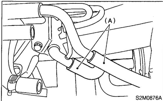
4) Remove bolt which installs pressure control solenoid valve holding bracket on body.
