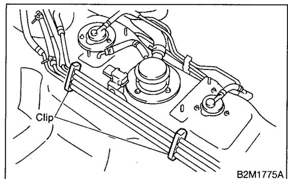
9) Move two fuel pipes to upper side, and remove bolt which install fuel tank pressure sensor to bracket.
