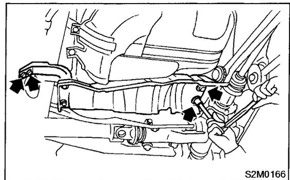
15) Install bolts which hold parking brake holding bracket.
