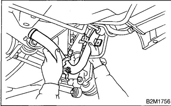
6) Disconnect evaporation hoses from shut valve.
