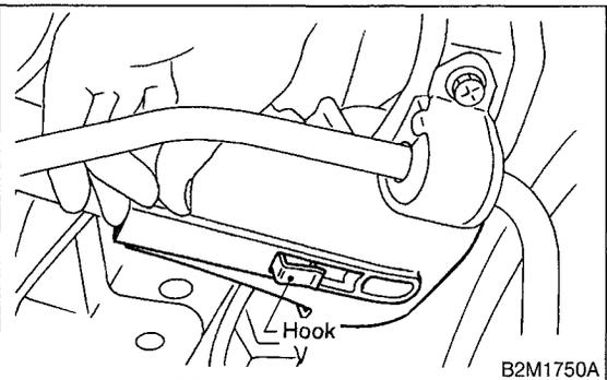
13) Disconnect evaporation hoses from pipes.
