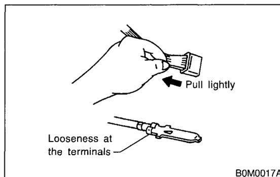
4) Insert the male pin of the connector into the female pin, then pull it out.
