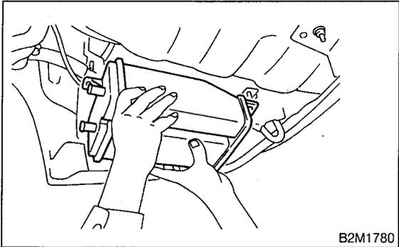
3) Disconnect evaporation hoses (A) from joint pipes.
