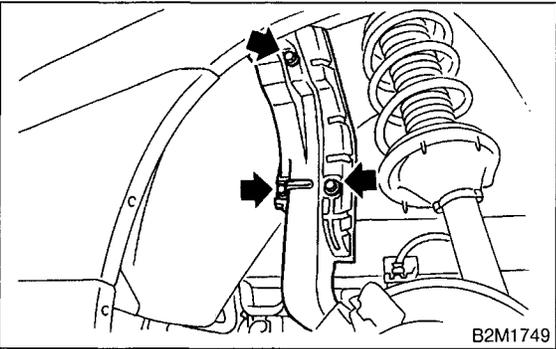
12) While releasing the under side of protector cover from hook, remove it.
