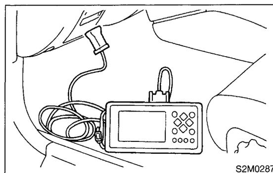
6) Turn ignition switch to ON (engine OFF) and Subaru select monitor switch to ON.
