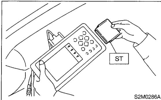
(2) Connect SUBARU SELECT MONITOR to the data link connector.
