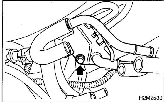
5) Disconnect connector from pressure control solenoid valve.
