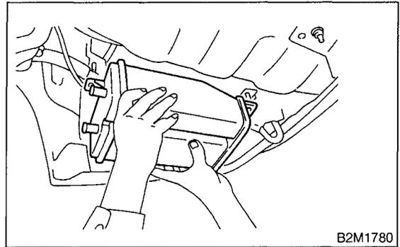
4) Disconnect connector from drain valve.
