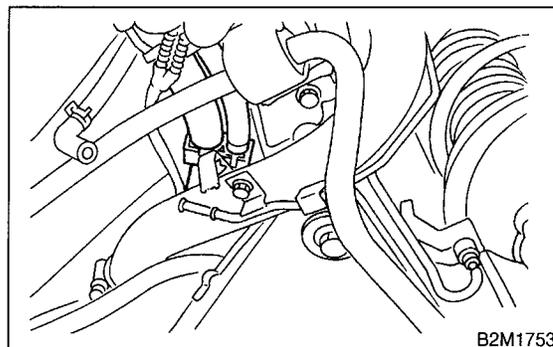
9) Connect evaporation hose to joint pipe.
