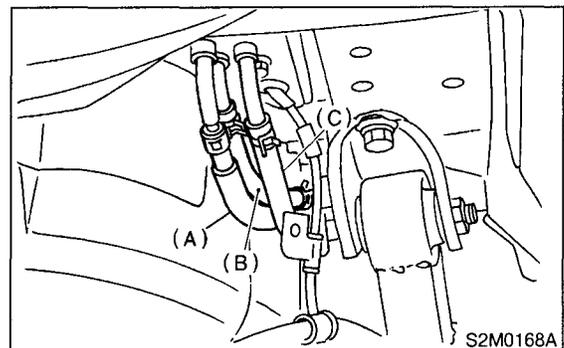
24) While holding fuel tank, remove bolts from bands and dismount fuel tank.
