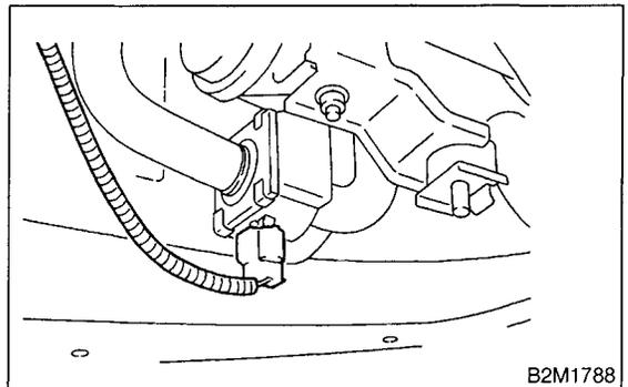
5) Disconnect evaporation hoses from drain valve.
