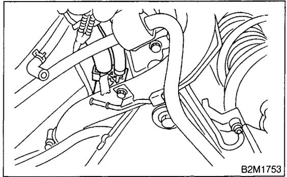
16) Disconnect evaporation hose from joint pipe.
