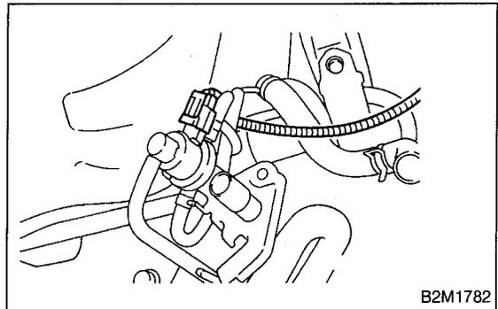
6) Disconnect two evaporation hoses from pressure control solenoid valve.
