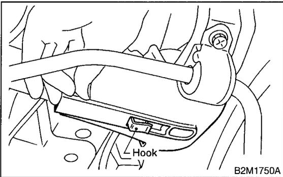
12) Tighten bolts which install protector cover on body.
