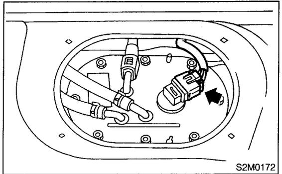
17) Install fuel sub meter unit, and connect connector and jet pump hose. <Ref. to 2-8 [W8A0].☆1>
