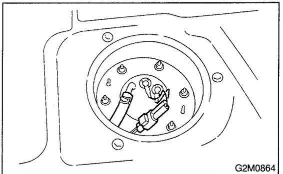
18) Connect connector to fuel pump relay.
