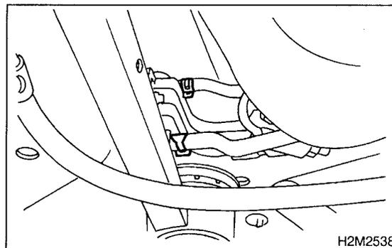
18) Remove bolts which hold parking brake cable holding bracket.
