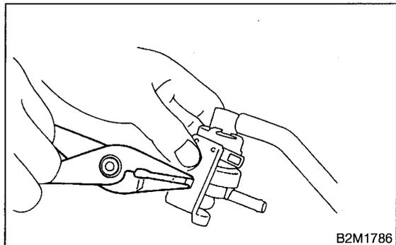
9) Disconnect vacuum hose from pressure control solenoid valve.
