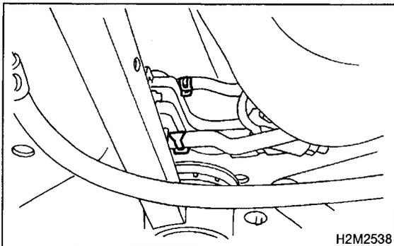
13) Install muffler assembly. <Ref. to 2-9 [W3A0].☆1>
