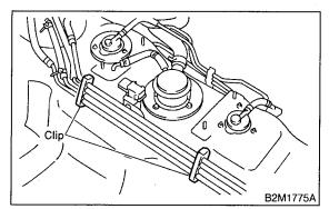
9) Move two fuel pipes to upper side, and remove bolt which install fuel tank pressure sensor to bracket.
