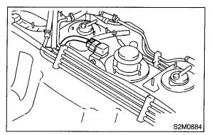
7) Disconnect connector from fuel tank pressure sensor.
