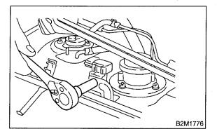
10) Move clip, and disconnect pressure hose from fuel tank.
