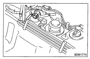
8) Release clips which hold fuel pipes onto fuel tank.
