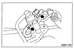
8) Remove pressure control solenoid valve from bracket.
