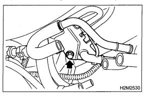
5) Disconnect connector from pressure control solenoid valve.
