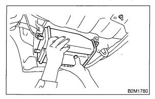
3) Disconnect evaporation hoses (A) from joint pipes.
