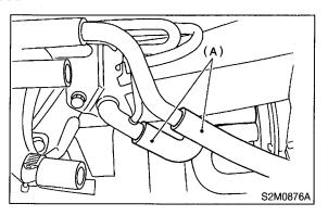
4) Remove bolt which installs pressure control solenoid valve holding bracket on body.
