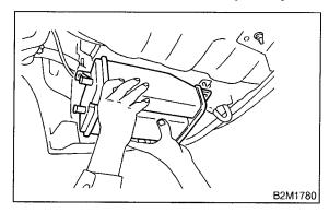
4) Disconnect connector from drain valve.
