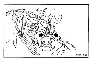
8) Remove nuts which install vent valve on fuel tank.
