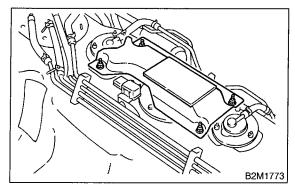
7) Move clips, and disconnect hoses from vent valve.
