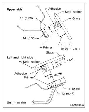
3) About one hour after installation, test for water leakage. Leave vehicle for 24 hours before using it.
