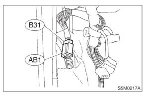
8) Detach clips from steering support beam and remove main harness.
