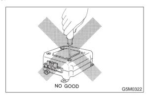
• If the airbag control module is deformed, or if water damage is suspected, replace the airbag control module with a new genuine part.
