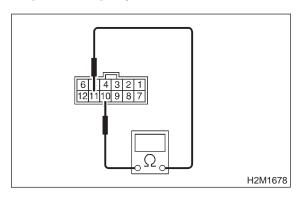
CHECK : Is the resistance less than 1  $\Omega$  in "2" range?
