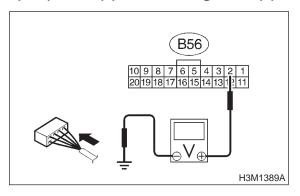
CHECK : Is the voltage less than 1 V in FWD
