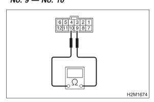
CHECK : Is the resistance less than 1  $\Omega$  in "R" range?
