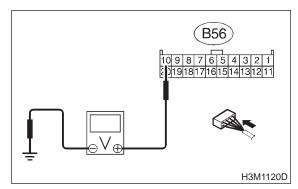
CHECK : Is the voltage less than 1 V in "R" range?
