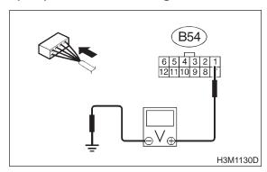
CHECK : Is the voltage less than 1 V in "D" range?
