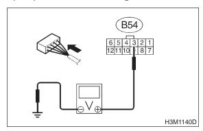
CHECK : Is the voltage less than 1 V in "2" range?
