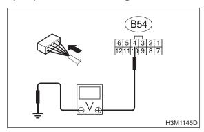
Is the voltage less than 1 V in "1" CHECK range?
