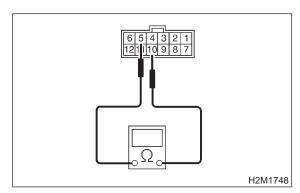
CHECK : Is the resistance less than 1  $\Omega$  in "N" range?
