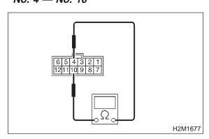
CHECK : Is the resistance less than 1  $\Omega$  in "3" range?
