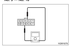
CHECK : Is the resistance less than 1  $\Omega$  in "1" range?
