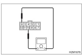
CHECK : Is the resistance less than 1  $\Omega$  in "D" range?
