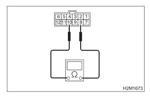
CHECK : Is the resistance less than 1  $\Omega$  in "P" range?
