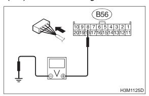
CHECK : Is the voltage less than 1 V in "N" range?
