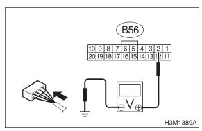
CHECK : Is the voltage more than 10 V in FWD switch while removing?
