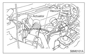
CHECK : Is there disconnection or cracks in vacuum hose?
