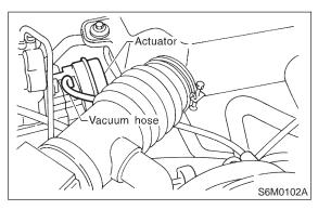
2) Connect vacuum pump as shown in figure.
