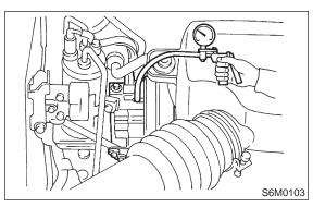
3) Make sure that cruise control cable moves smoothly and quickly when a vacuum pressure of 40.0 kPa (300 mmHg, 11.81 inHg) is applied to actuator.
