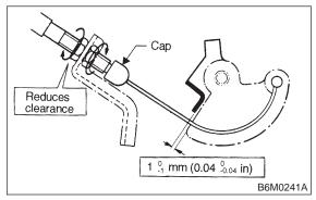
CHECK : Is throttle cam-to-lever clearance between 0 and 1 mm (0 and 0.04 in)?
