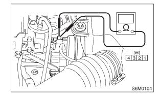
(CHECK) : Is resistance less than 69  $\Omega$ ?
