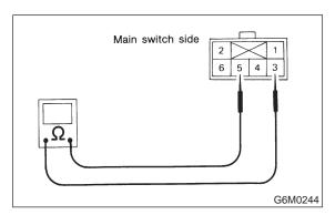
CHECK : Is resistance less than 1 MΩ? (When switch is OFF.)
