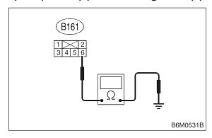
: Is resistance less than 10  $\Omega$ ? CHECK
