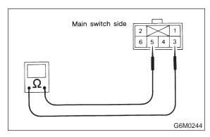
: Is resistance less than 10  $\Omega$ ? (When CHECK
