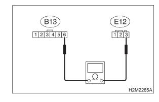
**CHECK** : Is the resistance less than 1  $\Omega$ ? **YES** : Go to step **8D10**.
