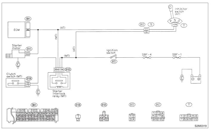
8. Diagnostics for Engine Starting Failure
