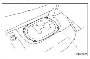
3) Disconnect connector from fuel pump.
