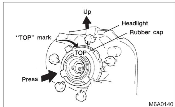
● To keep water out, correctly engage the groove portion of the rubber cap.
