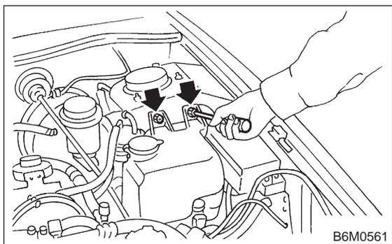
4) Disconnect washer tank connectors.
