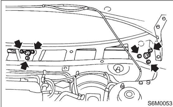
6) Remove wiper link from service hole in front panel.
