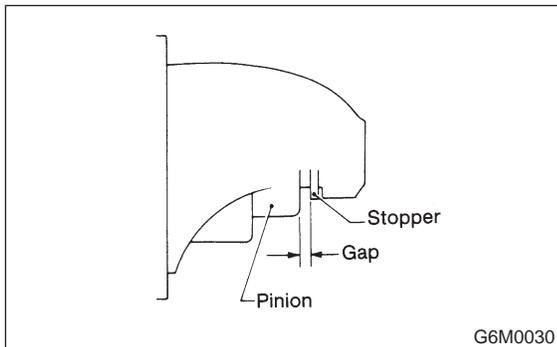
2) If motor is running with the pinion forced endwise on the shaft, disconnect connector from terminal M of switch assembly and connect terminal M to ground terminal (-) of battery with a lead wire. Next, gently push pinion back with your fingertips and measure pinion gap.
