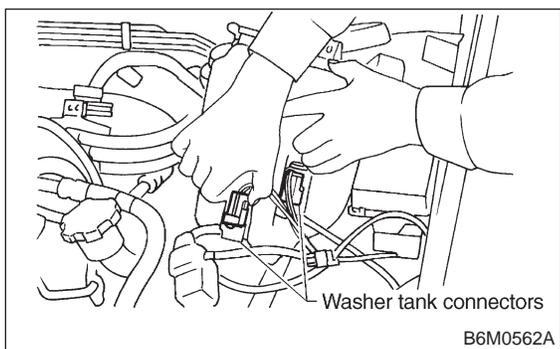
5) Move washer tank upward.
