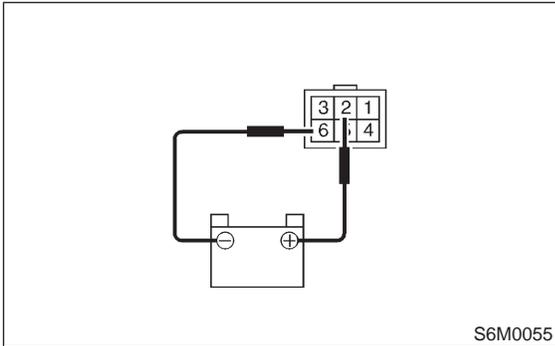
4) Reconnect battery and ensure that wiper motor stops at "AUTO STOP" after operating at low speed.
