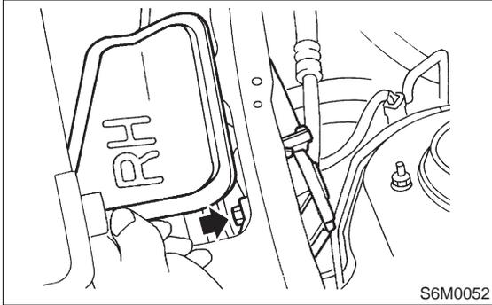
5) Remove bolts which secure sleeve unit.
