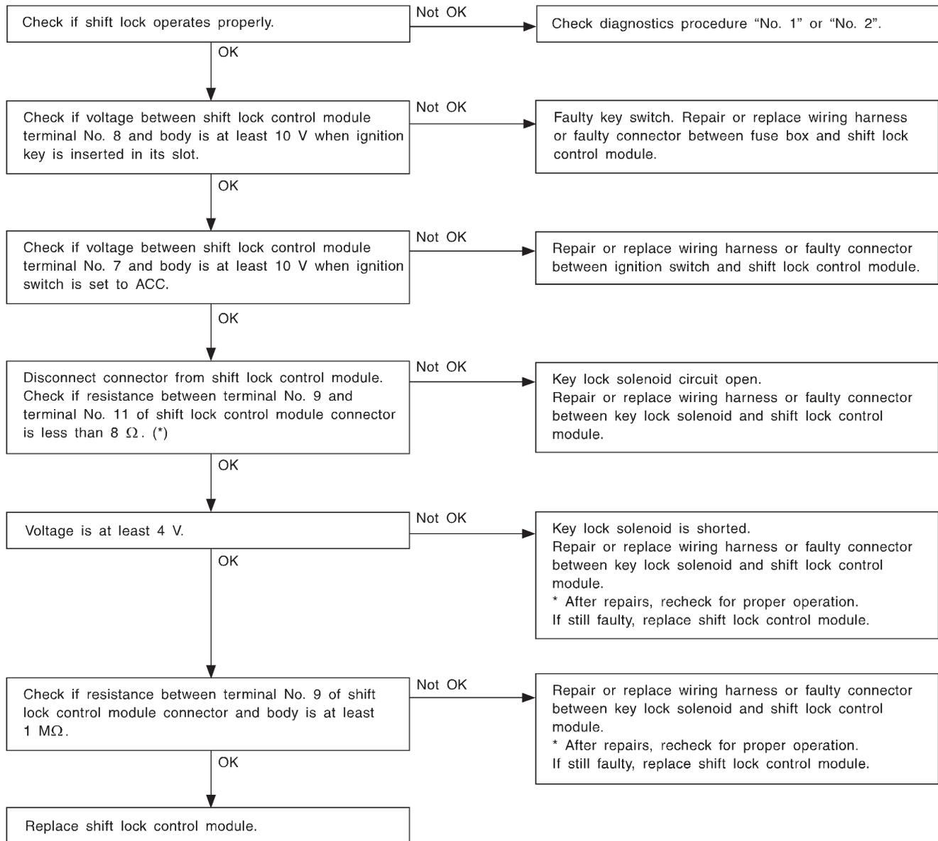
\*: When conducting operational checks of the key lock solenoid, do not apply 12 V to solenoid for more than one second, since this may break solenoid circuit.
