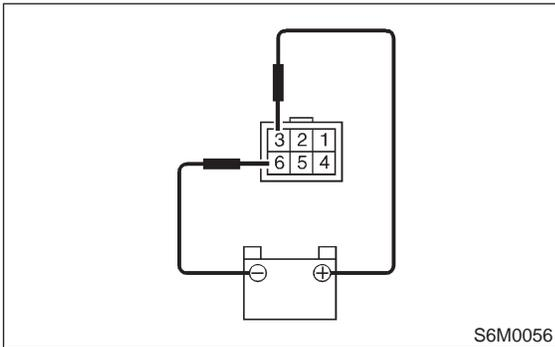
3) Check wiper motor for proper stoppage:
