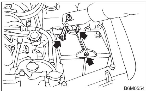
3) Remove washer tank mounting bolts.
