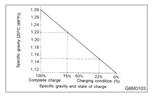
(2) Measuring the specific gravity of the electrolyte in the battery will disclose the state of charge of the battery. The relation between the specific gravity and the state of charge is as shown in figure.
