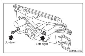
2) Look at the beam angle gauge (vertical movement). The bubble on the gauge should not deviate from the center of the gauge.
