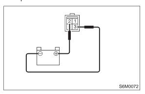
2) Check wiper motor for proper stoppage: After operating wiper motor, disconnect battery from wiper motor.
