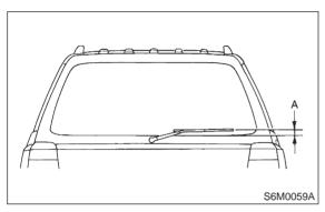
2) Adjust washer ejecting point on rear gate window as shown in figure when the vehicle stops.
