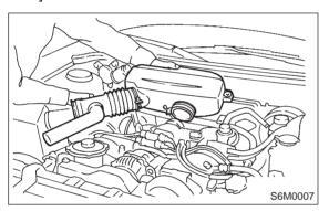
3) Disconnect connector from ignitor.
