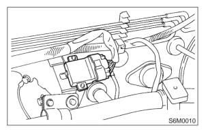
4) Remove screws which hold ignitor onto body.
