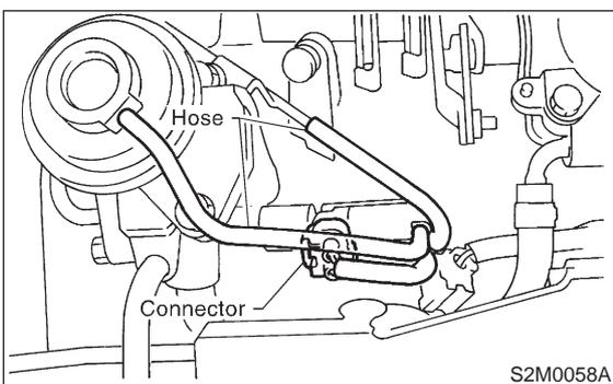
5) Remove bolt which installs EGR solenoid valve onto intake manifold.
