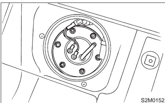
5) Remove sub fuel level sensor.
