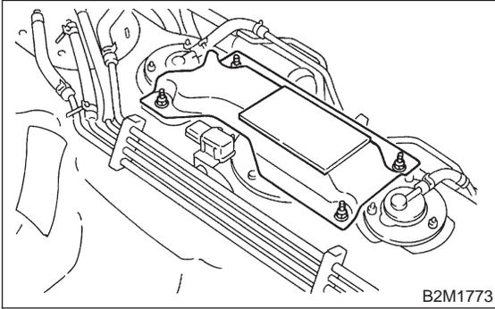
7) Move clips, and disconnect hoses from vent valve.
