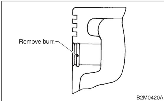
5) Check piston pin circlip for distortion, cracks and wear.
