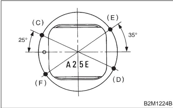
(5) Position the expander gap at 180° of the reverse side for the upper rail gap.
