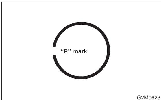
● The oil ring is a combined ring consisting of two rails and a spacer in between. When installing, be careful to assemble correctly.
