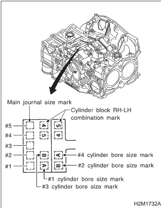
2) How to measure the inner diameter of each cylinder
