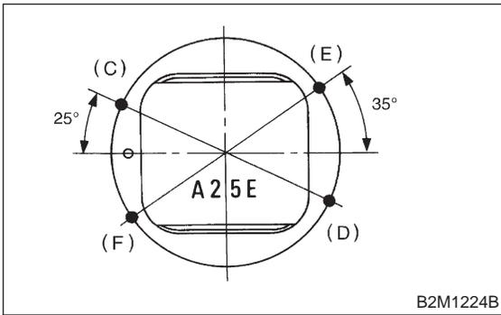
5) Install circlip.
