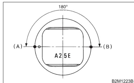
(3) Position the second ring gap at 180° on the reverse side for the top ring gap.
