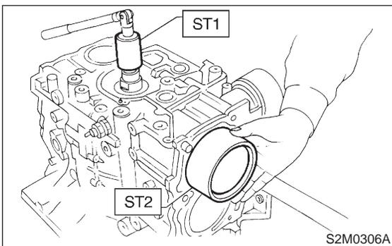
2) Installing piston pin
