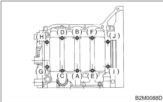
6) Tighten 8 mm and 6 mm cylinder block connecting bolts in alphabetical sequence shown in figure.
