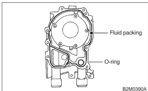
9) Install water pump and gasket.
