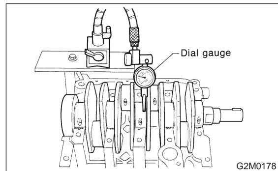
3) Inspect the crank journal and crank pin for wear. If not to specifications, replace bearing with an undersize one, and replace or recondition crankshaft as necessary. When grinding crank journal or crank pin, finish them to the specified dimensions according to the undersize bearing to be used.
