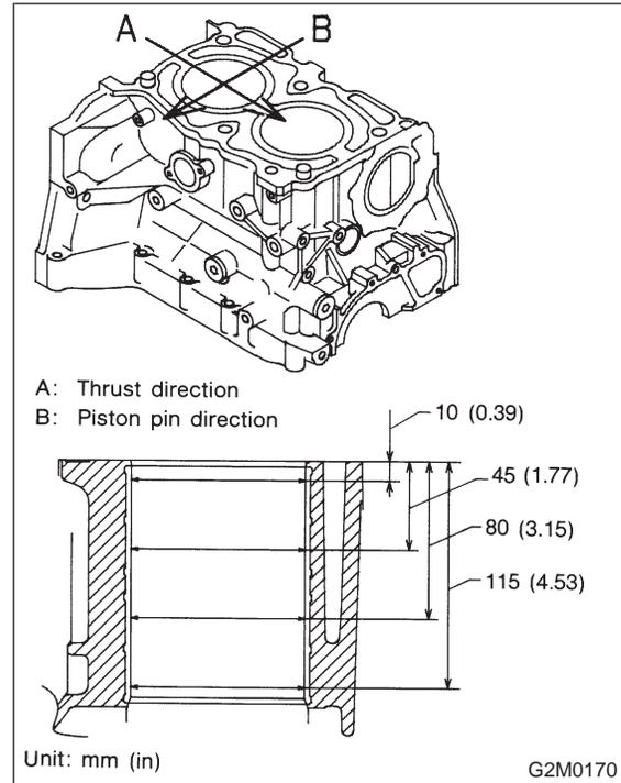
3) When piston is to be replaced due to general or cylinder wear, determine a suitable sized piston by measuring the piston clearance.
