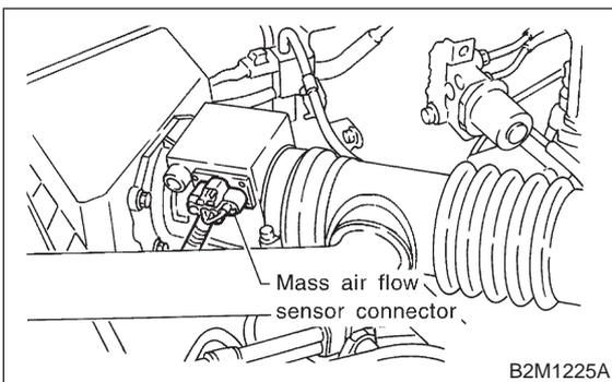
3) Loosen clamp which connects air intake duct to air intake chamber.
