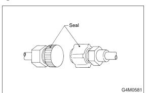
2) Visually inspect the O-ring surface, the O-ring mating surface, the threads and the connection points. If a defective part is found, replace it. The O-ring must sit square against the tube bead. If necessary, slide the O-ring into proper position with clean hands.
