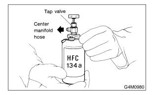
7) Disconnect the center manifold hose from the vacuum pump and connect the hose to the tap valve.
