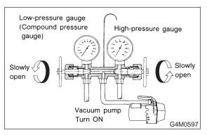
7) When the low-pressure gauge reaches approximately 66.43 kPa (498.3 mmHg, 19.62 inHg), slowly open the high-pressure manifold valve.
