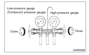
2) Attach the low-pressure manifold hose to the low-pressure service port on the vehicle. Check the low-pressure gauge. If more than 68.6 kPa (0.70 kg/cm<sup>2</sup>, 10 psi) is indicated, discharge the system prior to charging.
