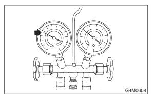
2) Keep the low side pressure below 276 kPa  $(2.81 \text{ kg/cm}^2, 40 \text{ psi})$  by using the low-pressure manifold valve to regulate the flow of refrigerant into the system.
