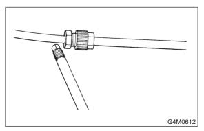
• Check the area where the two parts of the fitting join each other.
