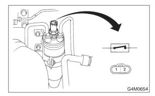
1) Remove cap from high-pressure line service valve, and connect gauge manifold to service valve.
