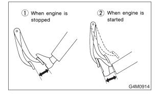
2) With brake pedal depressed, start engine.3) As engine starts, brake pedal should move slightly toward the floor. If no change occurs in the pedal height, brake booster is faulty.
