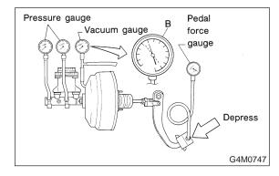
2) Stop engine and watch vacuum gauge. If the vacuum drop range is less than 3.3 kPa (25 mmHg, 0.98 inHg) within 15 seconds after stopping engine, brake booster is functioning properly. If defective, refer to "AIR TIGHTNESS CHECK". <Ref. to 4-4 [W6E2].>
