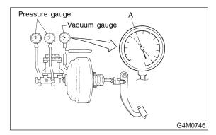
2) Stop engine and watch the gauge. If the vacuum drop range is less than 3.3 kPa (25 mmHg, 0.98 inHg) within 15 seconds after stopping engine, brake booster is functioning properly. If defective, the cause may be one of those listed below.
