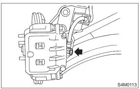
3) Secure middle fitting of brake hose to bracket at strut location using a clamp.
