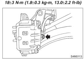
3) Secure middle fitting of brake hose to bracket at strut location using a clamp.
