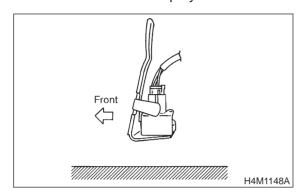
CHECK : Is the indicated reading 0.7±0.2 V when G sensor is inclined backwards to 90°?
