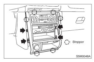
7) Remove control unit assembly from center console.
