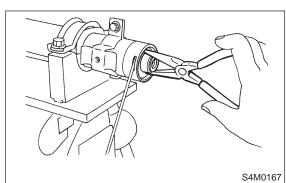
8) Fit mounting rubber onto rack housing.
