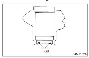
3) Attach ST2 to ST1, and press oil seal into place using a press.
