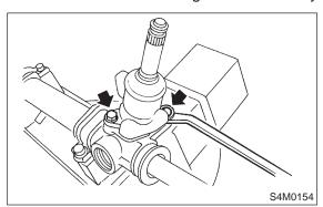
2) Carefully draw out input shaft and remove valve assembly.
