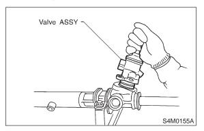
5) Tighten bolts alternately to secure valve assembly.
