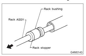
3) Remove rack bushing and rack stopper from rack assembly.
