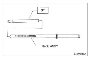
3) Apply genuine grease to teeth of thoroughly washed rack assembly, and fit ST over the toothed portion.
