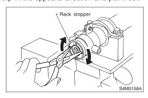
2) Pull rack assembly from cylinder side, and draw out rack bushing and rack stopper together with rack assembly.
