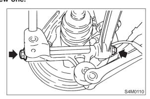
12) Disengage BJ from housing splines, and remove rear drive shaft assembly. If it is hard to remove, use STs.
