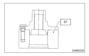
2) Remove foreign particles (dust, rust, etc.) from mating surfaces of hub and tone wheel, and install tone wheel to hub (only vehicle equipped with ABS).
