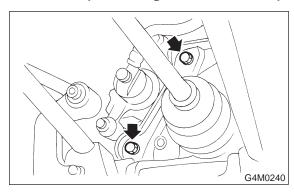
9) Install rear ABS sensor to back plate (only vehicle equipped with ABS).
