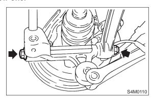
13) Disengage BJ from housing splines, and remove rear drive shaft assembly. If it is hard to remove, use STs.
