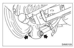
11) Remove bolts which secure lateral link assembly to rear housing.
