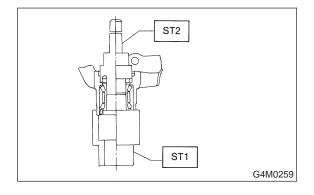
8) Using ST1 and ST2, press sub seal into place. ST1 927430000 HOUSING STAND ST2 927460000 OIL SEAL INSTALLER
