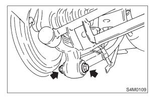
12) Remove bolts which secure lateral link assembly to rear housing.
