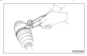
15) Tap on the clip with the punch provided at the end of ST.
