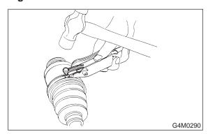
16) Cut off band with an allowance of about 10 mm (0.39 in) left from the clip and bend this allowance over the clip.
