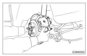
8) Connect rear housing assembly to trailing link assembly, and tighten self-locking nut.
