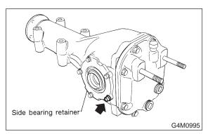
9) Remove axle nut and drive shaft. If it is hard to remove, use ST1 and ST2.
