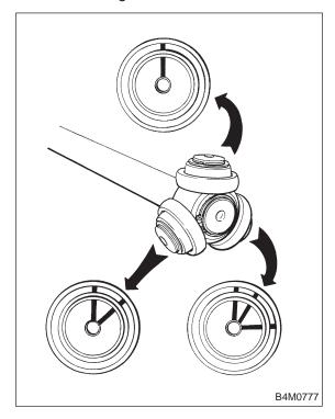
8) Align alignment marks on shaft and outer race, and install outer race.
