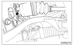
8) Remove front drive shaft assembly. If it is hard to remove, use ST1 and ST2.
