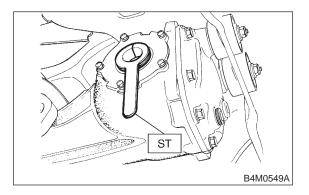
5) Insert DOJ spline end into bore of side oil seal, and remove ST.
