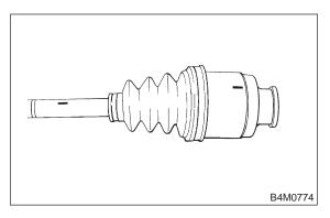
9) Install circlip in the groove on FTJ outer race.
