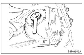
3) Insert DOJ spline end into bore of side oil seal, and remove ST.
