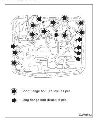
7) Remove shift solenoid assembly, and duty solenoid A.
