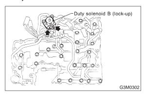
2) Install solenoid valves. Shift solenoid assembly, and duty solenoid A (line pressure).
