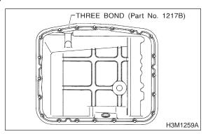
7) Install oil pan to transmission case.
