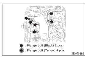
6) Remove control valve body and two brackets. Remove 6 long bolts (Black) and 11 short bolts (Yellow).
