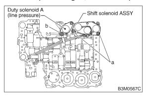
3) Install valve body and two brackets.
