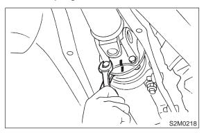
6) Install front exhaust pipe.
