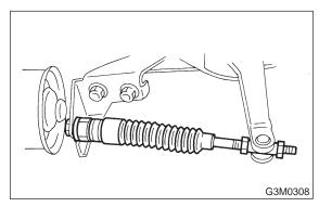
3) Install vehicle speed sensor 1.
