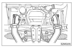
5) Remove propeller shaft and front exhaust cover.
