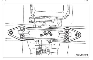
7) Remove vehicle speed sensor 1.
