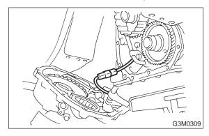
9) Remove duty solenoid C and transfer valve body from extension.
