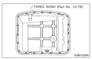
7) Install oil pan to transmission case.
