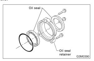
13) Attach the O-ring to the oil seal retainer with vaseline. Install the seal to the oil pump housing bore.
