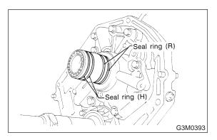
16) Install the rubber seal to the torque converter clutch case.
