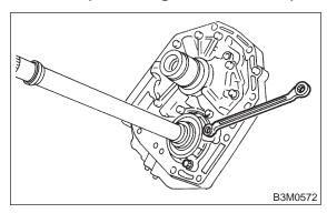
15) Apply vaseline to the groove on the oil pump cover, and install two (R) seal rings and two (H) seal rings.
