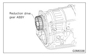
2) Remove the reduction driven gear.
