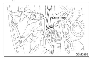
(2) Turning the case upside down, take out the one-way clutch inner race and spring retainer.
