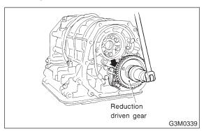
(2) Using the ST, extract the reduction driven gear.
