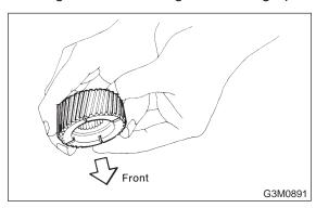
19) Install the front planetary carrier.
