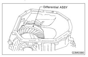
6) Install the circlip to the axle shaft, insert the shaft into the differential assembly, and tap it into position with a plastic hammer.
