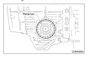
(6) After the "zero" state is established, back off the LH retainer 3 teeth and secure it with the lock plate. Then back off the RH retainer and retighten until it stops. Repeat this procedure several times. Tighten the RH retainer 1-3/4 teeth further. This sets the preload. Finally, secure the retainer with its lock plate.
