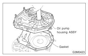
(4) Secure the housing with two nuts.
