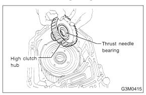
22) Install the high clutch assembly.
