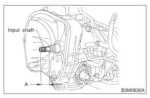
11) Install the torque converter clutch assembly.(1) Install the oil pump shaft to the torque converter clutch.
