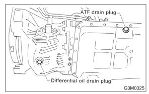
3) Remove the drain plug, and drain automatic transmission fluid (ATF). Tighten the plug temporarily after draining.
