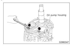
13) Loosen the brake band adjusting screw and take out the strut.
