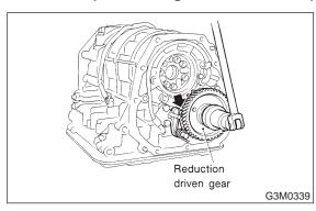
4) Install the reduction drive gear.
