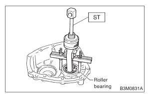
4) Take out the roller bearing outer race with ST. NOTE:
