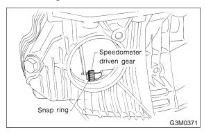
6) Tap out the speedometer shaft to the outside of the case, and remove the oil seal.
