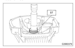
5) Install the differential assembly to the case, paying special attention not to damage the speed-ometer gears (drive and driven) and the inside of the case (particularly, the differential side retainer contact surface).
