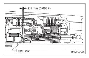
14) Assemble the overrunning clutch hub.
