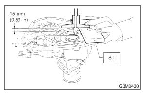
(2) Measure the distance " $\ell$ " from the transmission case mating surface to the reduction drive gear end surface with ST1 and ST2.
