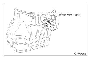
8) Install the oil seal and outer race (taper roller bearing) to the differential side retainer. Then screw in the retainer and the O-ring after coating the threads with oil.
