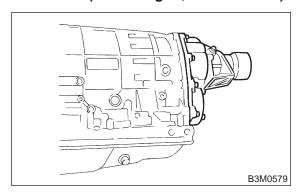
7) Install the vehicle speed sensor 1.
