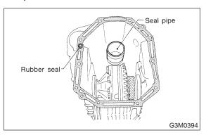
2) Install the torque converter clutch case assembly to the transmission case assembly, and secure with six bolts and four nuts.
