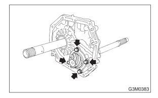
(3) Install the oil pump housing assembly to the torque converter clutch case, and secure evenly by tightening four bolts.
