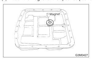
(2) Apply proper amount of liquid gasket (THREE BOND Part No. 1217B) to the entire oil pan mating surface.
