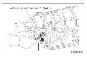
(2) While pulling the extension slightly, disconnect the connector for the duty solenoid C (transfer).
