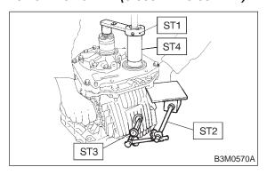
(8) Apply red lead evenly to the surfaces of three or four teeth of the crown gear. Rotate the drive pinion in the forward and reverse directions several times. Then remove the oil pump housing, and check the tooth contact pattern. If tooth contact is improper, readjust the backlash or shim thickness.
