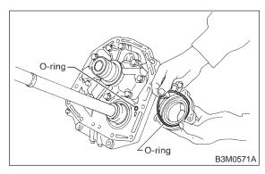
14) Install the oil seal retainer taking care not to damage the oil seal lips. Then secure with three bolts.
