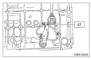
(2) With hole aligned, tighten three bolts to secure the inhibitor switch.
