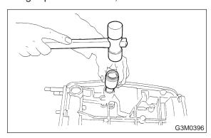
3) Install the manual plate and shaft, and secure with a spring pin.
