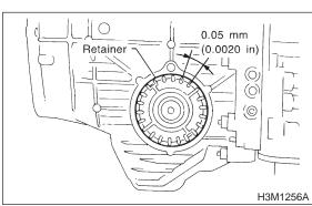
(7) Turn the drive pinion several rotations and check to see if the backlash is within the standard value with ST1, ST2, ST3 and ST4.
