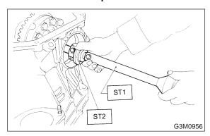
4) Remove the differential case assembly.
