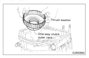
22) Take out the overrunning clutch hub, the thrust washer and the thrust bearing.
