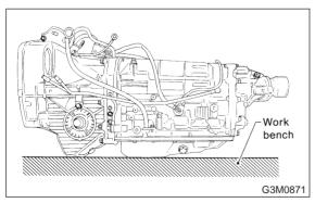
2) Remove the drain plug, and drain differential oil. Tighten the plug temporarily after draining.
