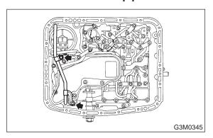
8) Disconnect the harness connectors for the solenoids and duty solenoids and the ground cord.
