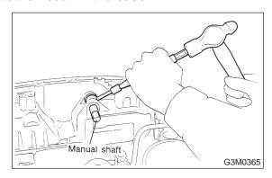
30) Remove the inhibitor switch.
