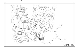
(3) Check the clearance. (Selection of retaining plate)
