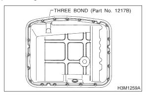
(3) Install the oil pan to transmission case.
