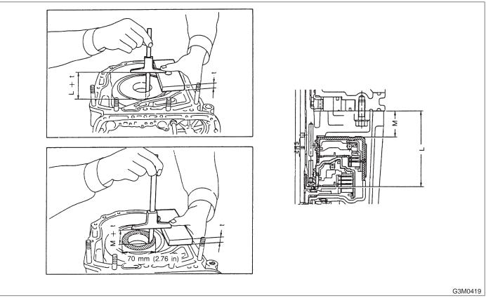
(2) Measure the distance from the oil pump housing mating surface to the top surface of the oil pump cover with needle bearing, and to the thrust surface of the reverse clutch.
