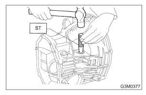
3) Install the speedometer driven gear to the speedometer shaft, and secure with a snap ring.
