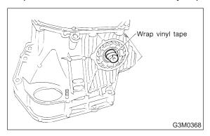
2) Remove the differential side retainer with ST. ST 499787000 WRENCH ASSY
