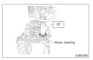
2) Using a plastic hammer, force-fit the oil seal.
