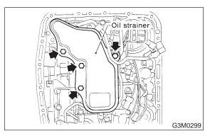
10) Remove the control valve body and the two brackets.
