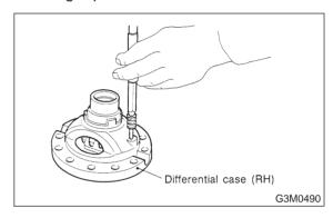
2) Install the washer and differential bevel gear to the differential case (LH). Then put the case over the differential case (RH), and connect both cases.
