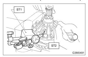
5) Install the speedometer drive gear. Then forcefit the taper roller bearing with a press and ST.
