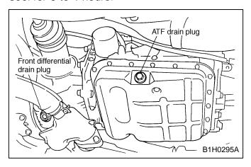
2) Reinstall drain plug after draining ATF, and tighten it to the specified torque.
