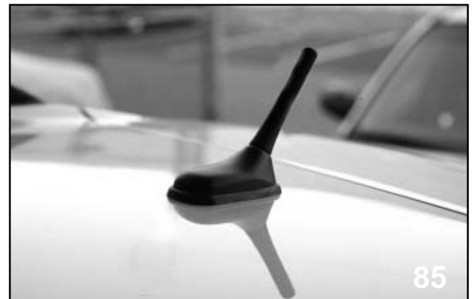
Cellular antenna and Global Positioning System (GPS) antenna.
