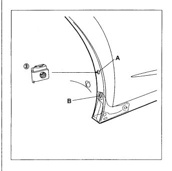
Slide rear plastic J nut (item<sup>®</sup>) into point A with hexagonal head away from mating surface.
