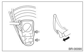
5) Close the outlet plug with your finger, and release the brake pedal.
