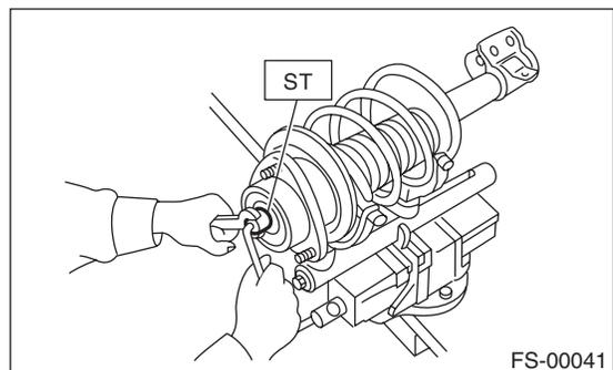
10) Loosen the coil spring carefully.
