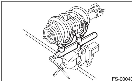
2) Using the ST, remove the self-locking nut.
