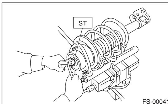
3) Remove the strut mount, upper spring seat and rubber seat from the strut.
