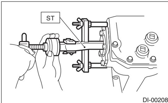
9) Install a new side oil seal using the ST.
