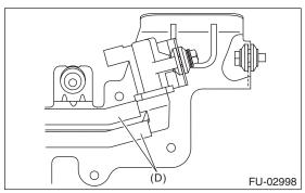
7) Remove the wastegate control solenoid valve from the bracket.
