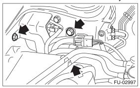
6) Disconnect pressure hose (D) from the wastegate control solenoid valve.
