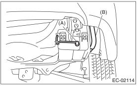
7) Remove the canister from the body.
