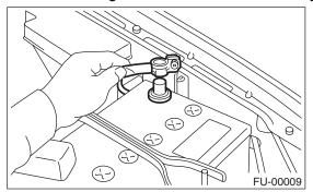
2) Disconnect the connector and evaporation hoses of purge control solenoid valve, and then remove the purge control solenoid valve.
