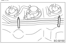
5) Remove the bolt and nut which secures the fuel tank pressure sensor to the bracket.
