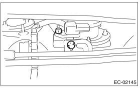
6) Disconnect the pressure hose from the fuel tank pressure sensor.
