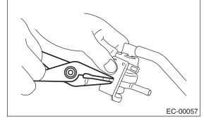
10) Disconnect the hose from the pressure control solenoid valve.
