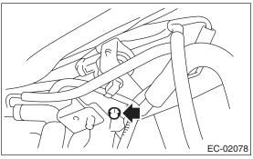
6) Remove the pressure control solenoid valve and the bracket as a unit.
