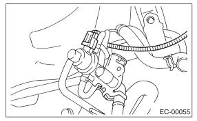
8) Disconnect the two evaporation hoses from the pressure control solenoid valve.
